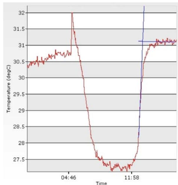
An example of a dryout curve from the DRT-201's connected software that provides a useful measurement of a fabric's wicking performance.
