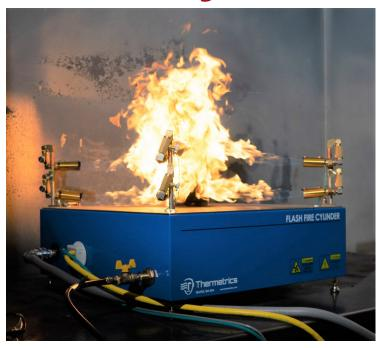
This innovative benchtop instrument is designed to provide effective 3D sample evaluation and to bridge the gap between flat-specimen TPP testing and full-garment Flame Manikin tests.
