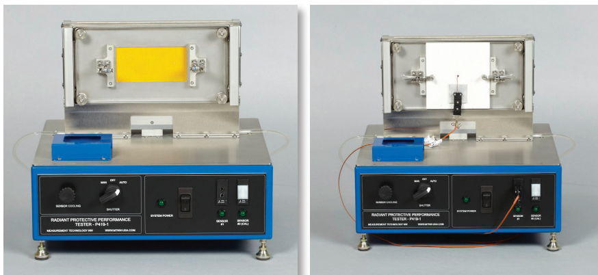
RPP Device with sample tray in place (left) and with sensor in place (right)
