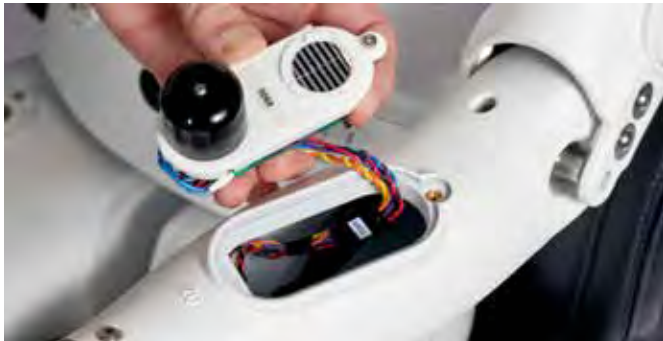
Environmental sensor module measures air speed, temperature, dual-spectrum heat flux, and relative humidity.
