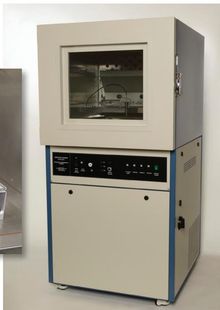
**The Sweating Guarded Hotplate, or "Skin Model", is used to produce accurate, repeatable measurements of thermal resistance ( $R_{ct}$ ) and vapor permeability ( $R_{et}$ ) for textiles as per ISO 11092, ASTM F1868, and ASTM D1518 (Option II).**
